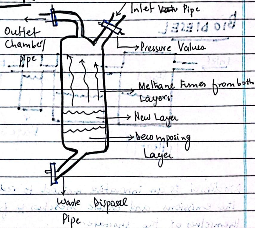
Biogas is an environmentally friendly solution to get self-sufficiency at energy production. It works
