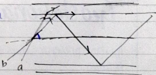
Now if ray 'a' is thrown it reaches the core-cladding boundary and it refracts at an angle because it was not thrown at the critical angle while ray 'b' which is thrown at the critical angle will reflect back at a certain angle and will continue to zigzag along the optic fiber until it reaches its destination
