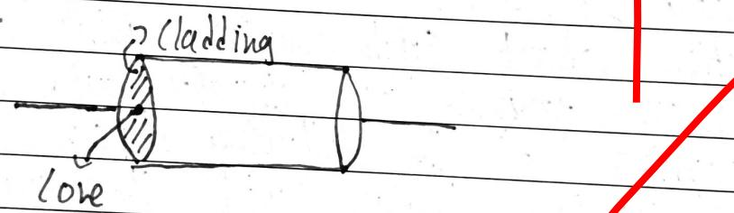
The optical fibre works by achieving total internal reflection of light. This usually occurs at core-cladding boundary.
