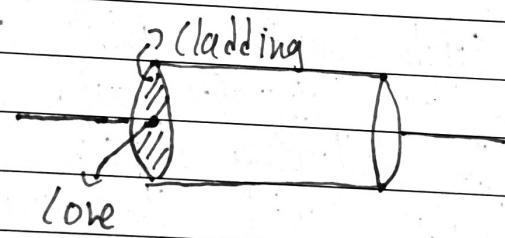
The optical fibre works by achieving total internal reflection of light. This usually occurs at core-cladding boundary.
