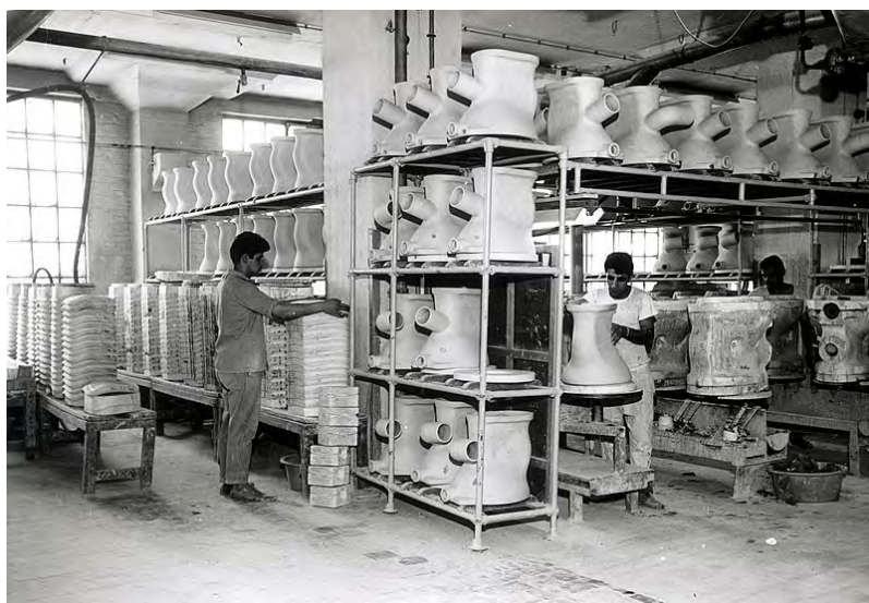
Fig. 2: Factory workers working on bathroom fixtures to be baked in tunnel ovens at Royal Sphinx in Maastricht, the Netherlands (ca. 1960–ca. 1970), CC BY 3.0, Wikimedia, https://commons.wikimedia.org/wiki/File:Sphinx_sanitairproductie,_jaren_60_%285%29.jpg .
