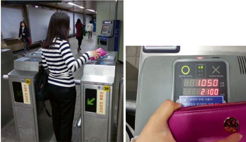
Figure 11.5 The credit-based transportation card displays the fare and accumulated charges for the current month at the ticket gate (Photos by J. K. Lee)
