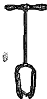
FIG. 111. Post-hole auger. Small-diameter augers of this type are used for studying the distribution of irrigation water in soil. (Courtesy Iwan Brothers.)
