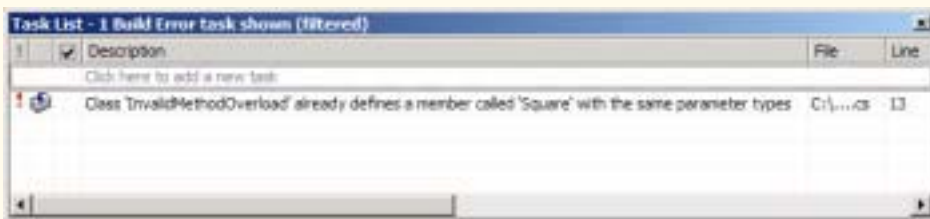
Fig. 6.19 Syntax error generated from overloaded methods with identical parameter lists and different return types.
