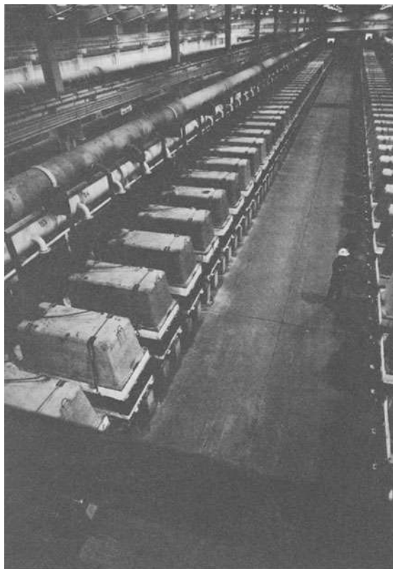
Fig. 12.12. A series of Diamond Shamrock cells. (Courtesy Diamond Shamrock Corporation.)
