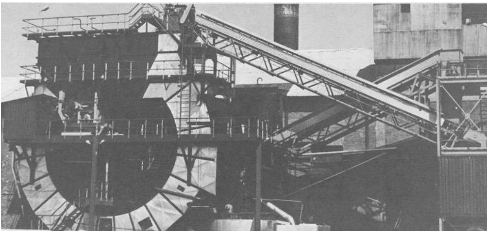
Fig. 9.8. Continuous ring type total maseration sugarcane diffuser. (Courtesy Sucatlan Engineering, Paris.)
