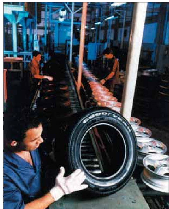
A GOODYEAR ASSOCIATE INSPECTS A RADIAL TIRE AT THE SAO PAULO, BRAZIL, FACTORY BEFORE MOUNTING IT ON THE WHEEL. GOODYEAR PRACTICES BOTH VISUAL AND INTERNAL INSPECTIONS OF TIRES, EVEN PULLING SOME TIRES FROM THE PRODUCTION LINE TO BE X-RAYED. QUALITY CONTROL ENGINEERS ALSO REGULARLY CUT APART RANDOMLY CHOSEN TIRES TO STUDY VARIOUS DETAILS THAT MAY AFFECT PERFORMANCE, RIDE, OR SAFETY.
