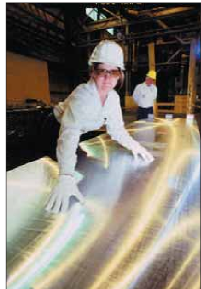
ALUMINUM SHEETS ARE EXAMINED UNDER QUALITY CONTROL LIGHTS ON THE ALUMINUM PRODUCTION LINE AT THE ALCOA SZÉKESFEHÉRVÁR, HUNGARY, EXTRUSION PLANT.
