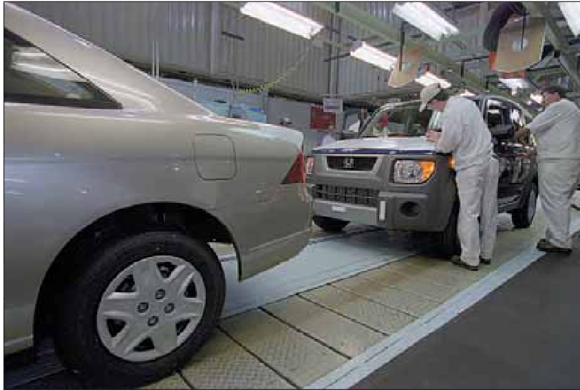
HONDA'S NEW MANUFACTURING SYSTEM ENABLES PRODUCTION OF ACCORD SEDANS ON THE SAME ASSEMBLY LINE THAT PRODUCES CIVIC COMPACTS AND ELEMENT LIGHT TRUCKS AT THIS EAST LIBERTY, OHIO, PLANT.
