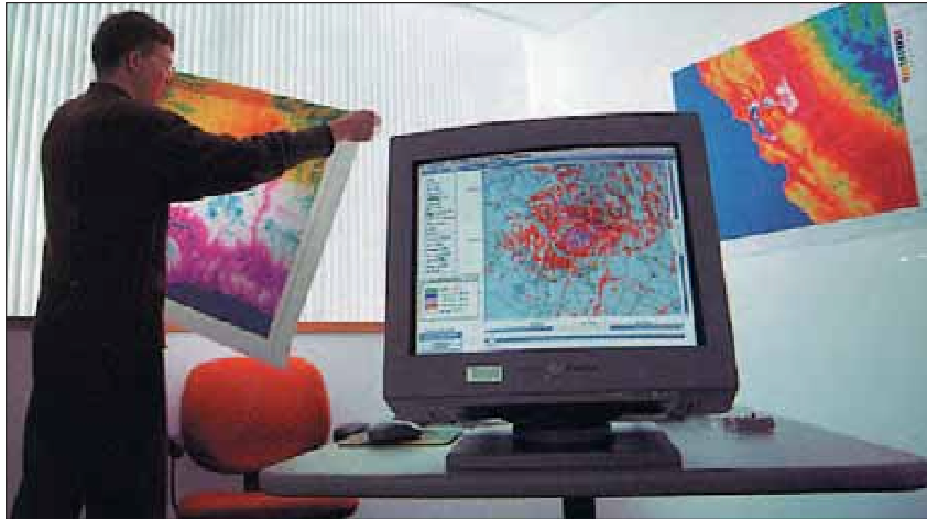
A GTE LABORATORIES ENGINEER EXAMINES A PRINT GENERATED BY GRANET, A GRAPHICS-BASED SOFTWARE TOOL DEVELOPED BY GTE TO HELP ENGINEERS WORLDWIDE PLAN CELLULAR NETWORKS AND FORECAST THEIR PERFORMANCE.
