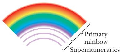
Figure 35-5 A primary rainbow and the faint supernumeraries below it are due to optical interference.
