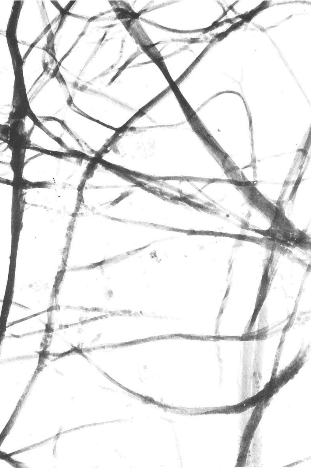
Silk fibers as photographed with the electron microscope. The magnification here is about 6,000 times.
