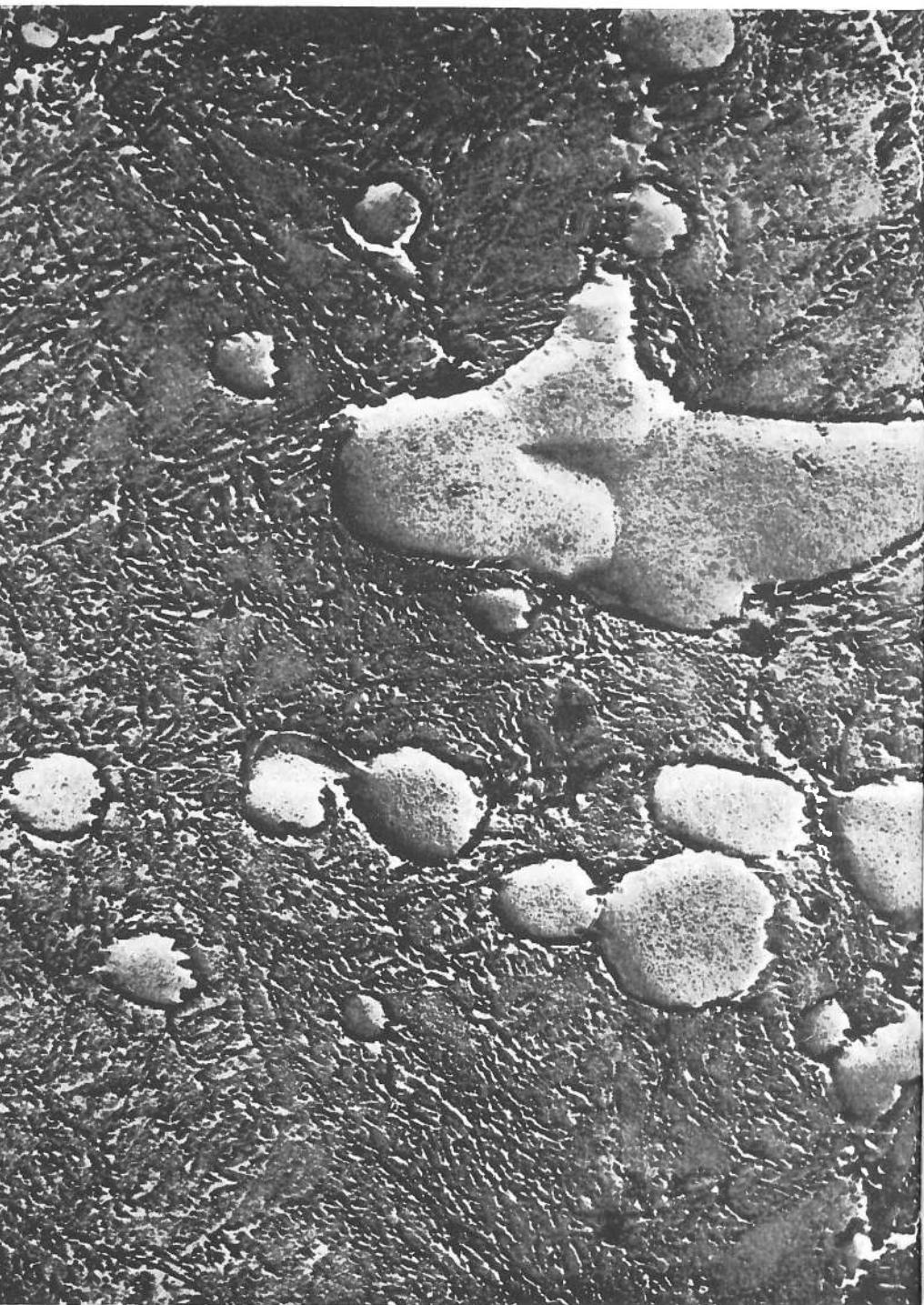
Electron micrograph of the surface of a piece of etched steel.
