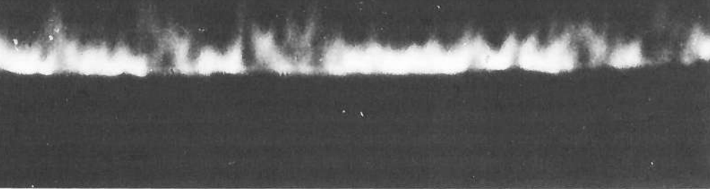
Magnetic domains photographed with an electron microscope by a special technique. The line of light shows the fine edge of a thin, magnetized piece of steel; the faint areas represent the deflection of electrons by the magnetic domains.
