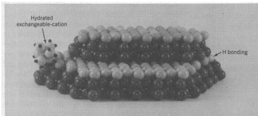
FIGURE 10.13 Model of kaolinite showing two offset layers. The upper layer surfaces are composed of hydroxyls (light-colored). These hydroxyl are bonded by the hydrogen of the hydroxyl to the oxygen of adjacent layers, producing a nonexpanding clay. Cation exchange capacity is low and originates at the edges due to deprotonation of exposed hydroxyls. A hydrated cation is adsorbed to such a cation exchange site.
