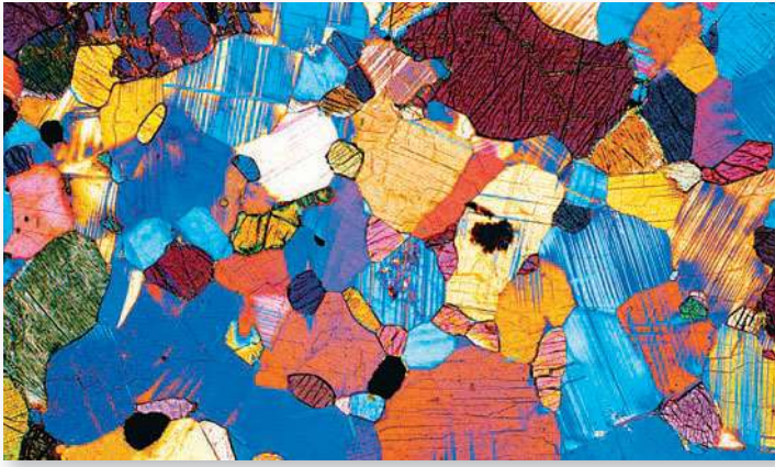
FIGURE 14.7 Crystals of different minerals create beautifully colored patterns in a rock sample seen in a polarizing microscope.
