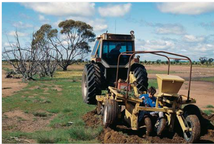
FIGURE 13.7 Mechanical planters can plant thousands of trees per day.
