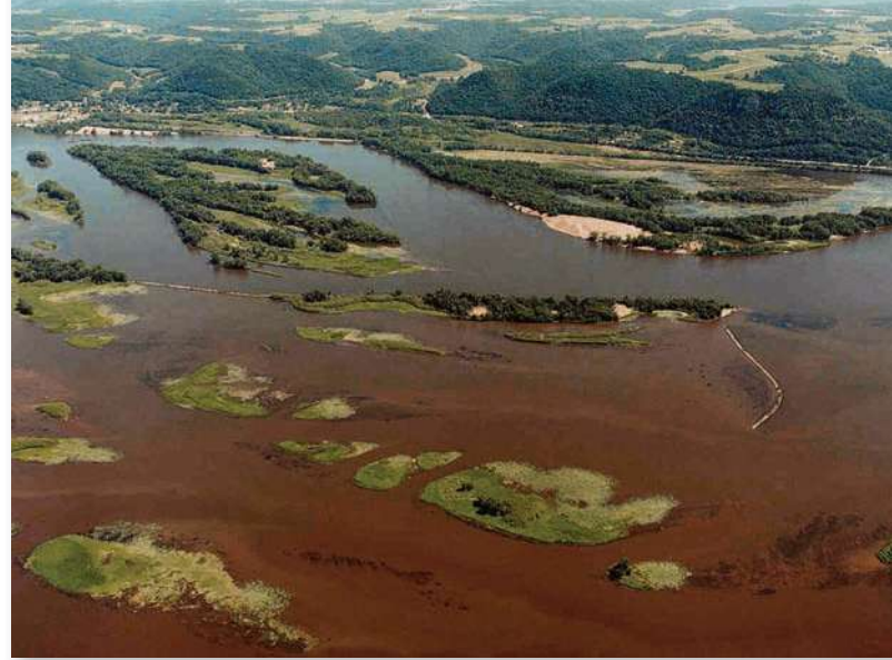
FIGURE 13.22 Dams on the upper Mississippi River have created a series of large lakes. Currents created by wind, floods, and river traffic keep the soft sediment stirred up so that wetland plants can't take root. To restore these backwaters, the Army Corps is experimenting with wing dams (see thin white lines between islands) that will allow the mud to solidify and turn into marshlands.
