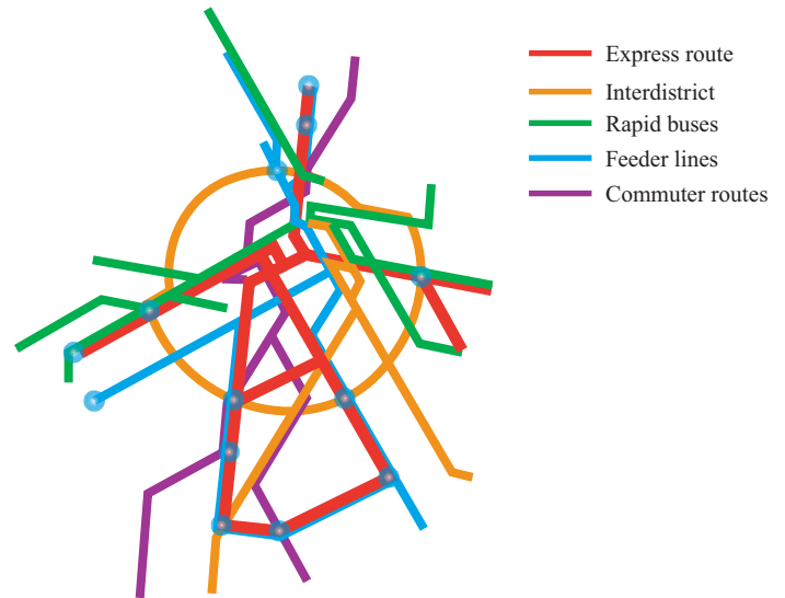
FIGURE 22.16 Curitiba's transit system has more than 340 interlinked bus routes. Neighborhood feeder lines connect to high-volume, express buses running on dedicated busways. Interdistrict routes carry passengers between suburbs, while specialized commuter routes carry workers directly from distant neighborhoods to the city center. Altogether this system moves more than 1.9 million people per day, or more than 75 percent of all personal transportation in the city.
