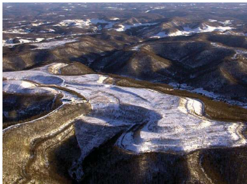
FIGURE 14.13 Mountaintop removal mining is a relatively new, and deeply controversial, method of extracting Appalachian coal.
