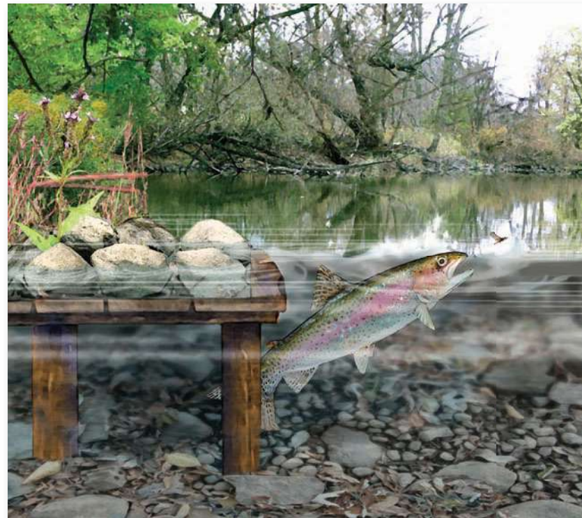
FIGURE 13.31 A lunker structure is a multilevel wooden framework that rests on the stream bottom and can be anchored to the shore. The top of the box is covered with rock, soil, and vegetation. Openings in the structure provide hiding places for fish.
