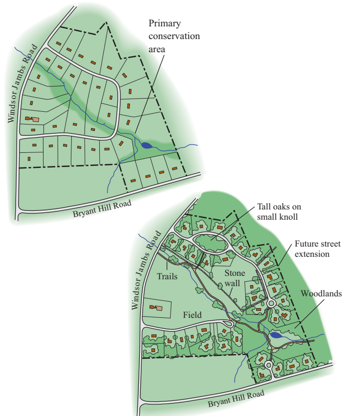
FIGURE 22.22 Conventional subdivision ( top ) and an open space plan ( bottom ). Although both plans provide 36 home sites, the conventional development allows for no public space. Cluster housing on smaller lots in the open space design preserves at least half the area as woods, prairie, wetlands, farms, or other conservation lands, while providing residents with more attractive vistas and recreational opportunities than a checkerboard development.
