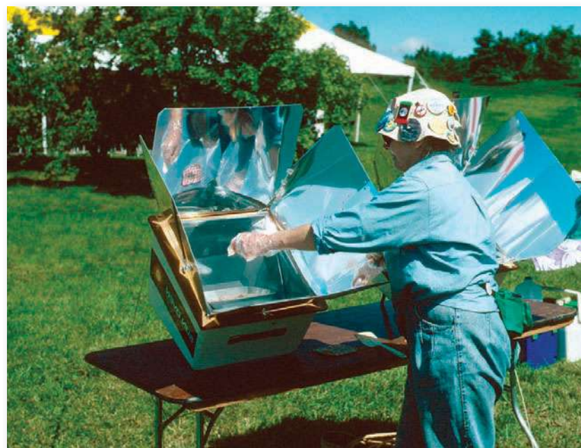
FIGURE 20.11 A simple box of wood or cardboard, plastic, and foil can help reduce tropical deforestation, improve women's lives, and avoid health risks from smoky fires in developing countries. These inexpensive solar cookers could revolutionize energy use in developing tropical countries.
