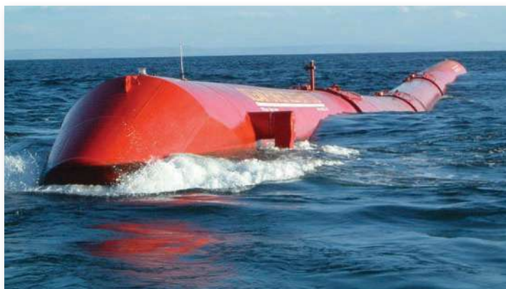
FIGURE 20.31 The Pelamis wave converter (named after a sea snake) is a 125 m long and 3.5 m diameter tube-hinged, so it undulates as ocean swells pass along it. This motion drives pistons that turn electrical generators. Energy experts calculate that capturing just 1 to 2 percent of global wave power could supply at least 16 percent of the world's electrical demand.
