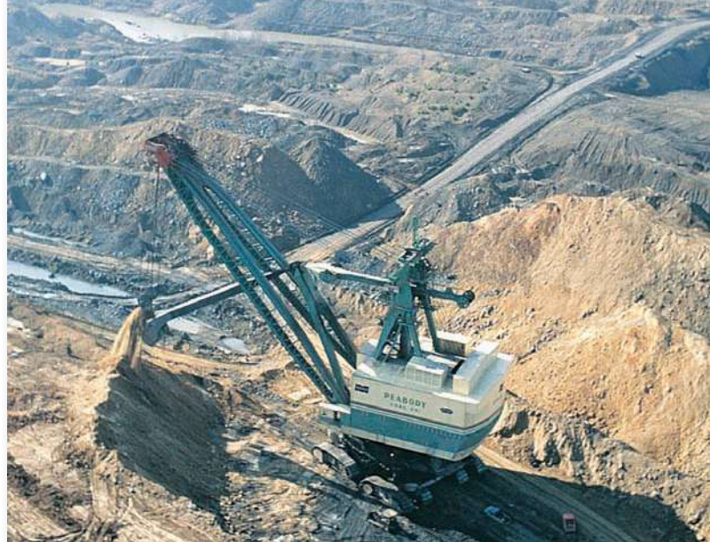
FIGURE 14.12 Some giant mining machines stand as tall as a 20-story building and can scoop up thousands of cubic meters of rock per hour.
