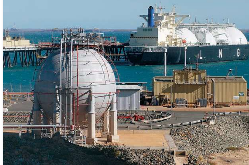
FIGURE 19.16 As domestic supplies of natural gas dwindle, the United States is turning increasingly to shipments of liquefied gas in specialized ships, such as this one at an Australian terminal. An explosion of one of these ships would release about as much energy as a small atomic bomb.
