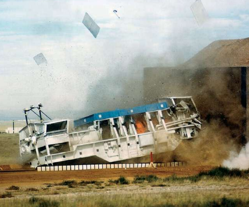
FIGURE 19.27 A test railcar carrying a spent nuclear fuel shipping cask slams into a concrete wall at 130 km/hr (81 mph). The cask survived without injury. Even so, many people don't want nuclear waste shipped through their city. Would you?
