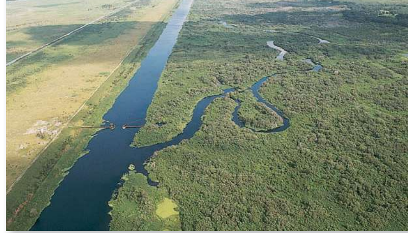
FIGURE 13.25 The naturally meandering Kissimmee River (right channel) was straightened by the Army Corps of Engineers (left) for flood control 30 years ago. Now the Corps is attempting to reverse its actions and restore the Kissimmee and its associated wetlands to their original state.
