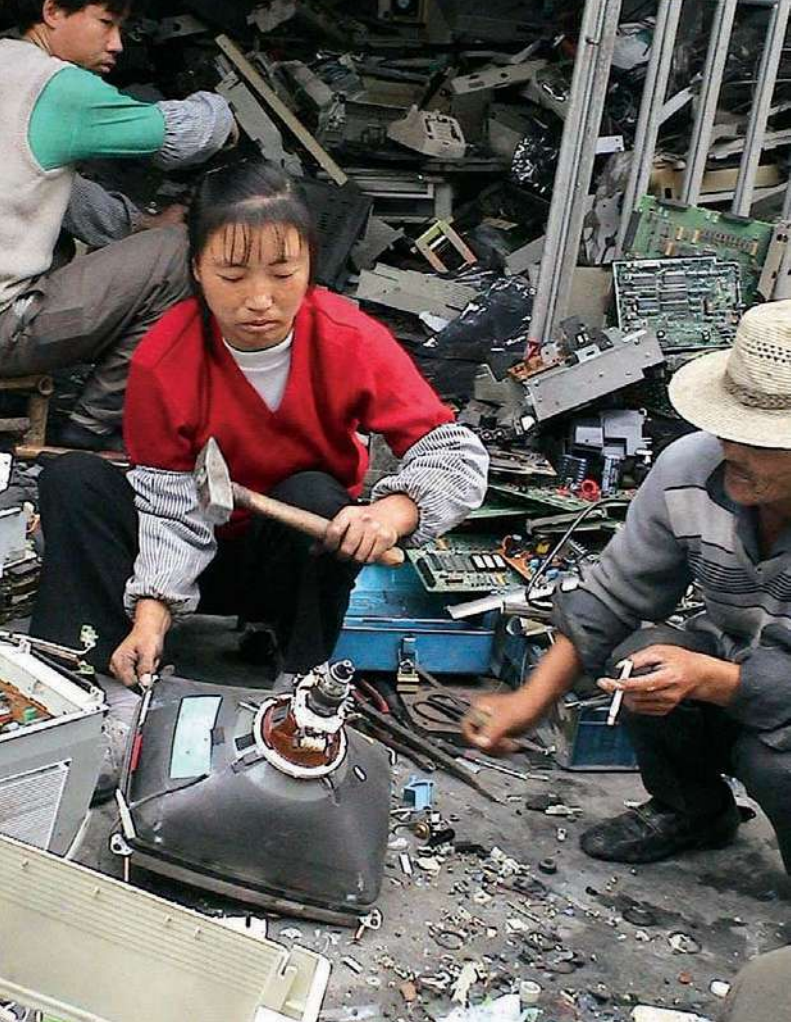
FIGURE 21.6 A Chinese woman smashes a cathode ray tube from a computer monitor in order to remove valuable metals. This kind of unprotected demanufacturing is highly hazardous to both workers and the environment.
