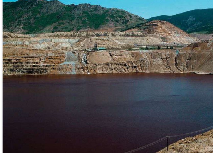
FIGURE 13.34 The Berkely mine pit in Butte, Montana, may be the most toxic water body in the United States. Water entering the pit is now being treated and eventually there may be an effort to pump water out of the pit and decontaminate it, but the pit itself will probably never be filled in.
