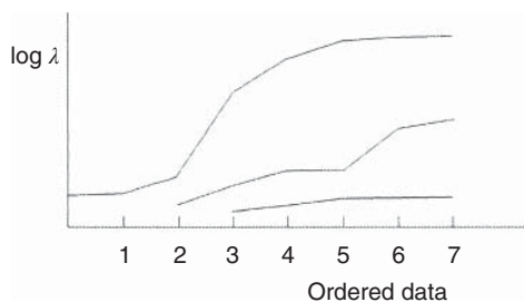
Figure 5.11 Schematic representation of evolving eigenvalues, \lambda , in dependence on intrinsically ordered data.
