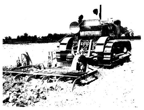
Figure 5-6. The chisel, a tool for deep tillage. [Courtesy Caterpillar Tractor Co.]
