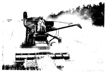
Figure 8-4. Combine with pick-up attachment threshing from windrow. [Courtesy John Deere & Co.]
