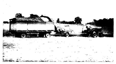
Figure 8-12. Forage harvester for gathering green material for silage or soilage. [Courtesy Allis-Chalmers Manufacturing Co.]
