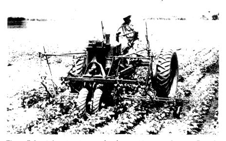
Figure 5-8. Cultivating six rows of soybeans with sweeps that cut off weeds about 1 inch below the soil surface. [Courtesy International Harvester Co.]
