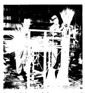
Figure 13–10. Making brooms on a homemade foot-treadle machine. The brush is wound onto the handle with wire at the left. A broom is handstitched in a clamp at the right. Power winders and mechanical sorting, trimming, and stitching machines are used in commercial broom factories.
