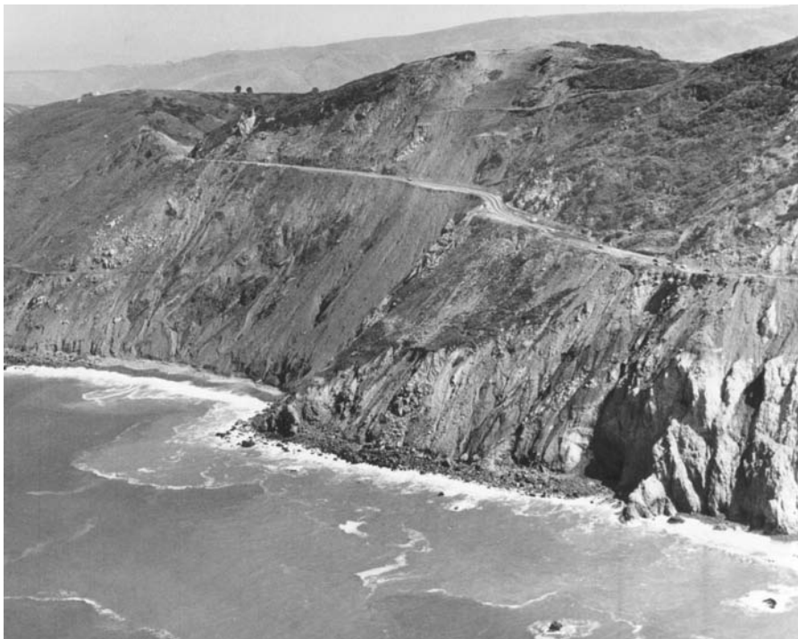
Figure 77 Devils Slide caused by storm waves that continue to erode the base of the cliff, San Mateo County, California.
