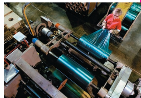
Cellophane on rollers at a manufacturing plant.
