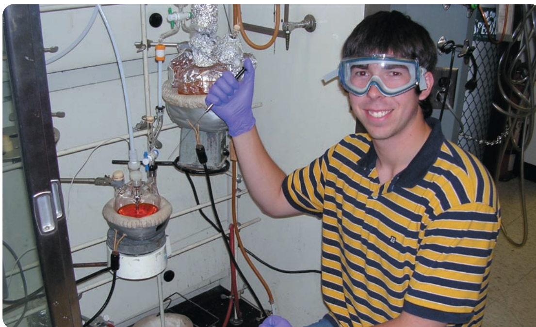
Some reactions with carbonyl compounds involve reagents that we transfer by syringe to keep them away from moisture and air.
