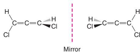
Figure 5.22 Enantiomeric forms of 1,3-dichloroallene. These two molecules are nonsuperposable mirror images of each other and are therefore chiral. They do not possess a tetrahedral atom with four different groups, however.
