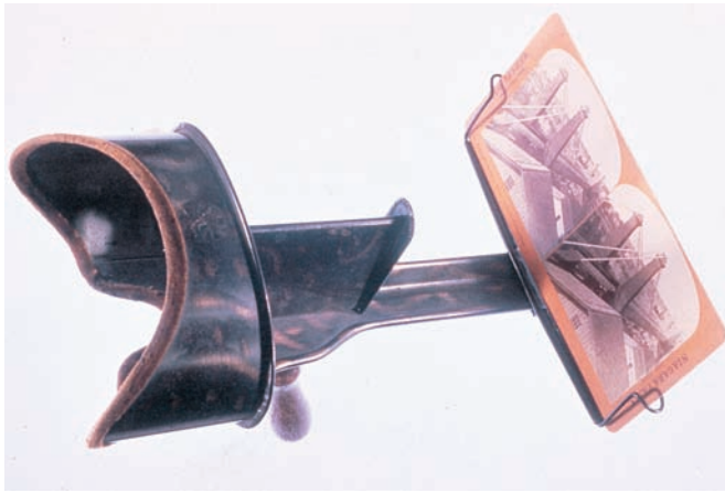
The Holmes-Bates stereoscope, invented by Oliver Wendell Holmes in 1861 and manufactured by Joseph Bates, creates a vivid perception of depth.
