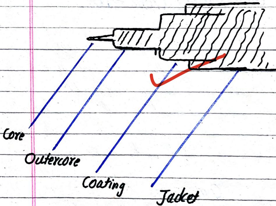
Figure 0.2 diagram of Optic fiber
