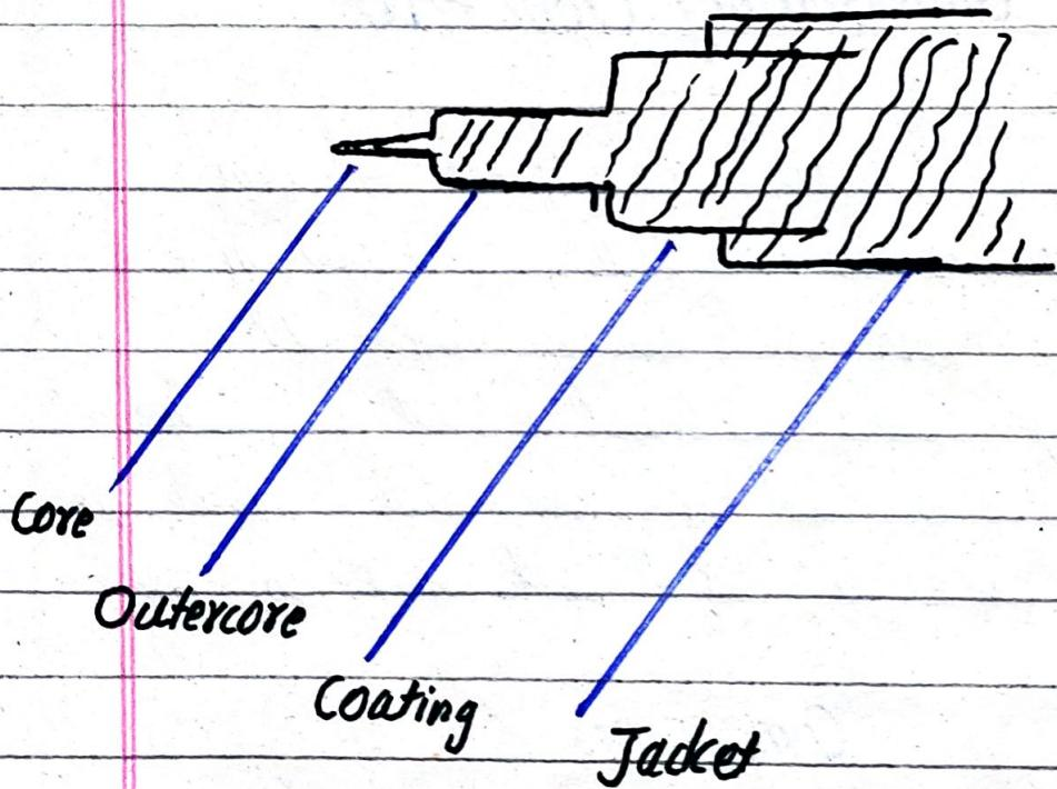
Figure 0.2 diagram of Optic fiber
