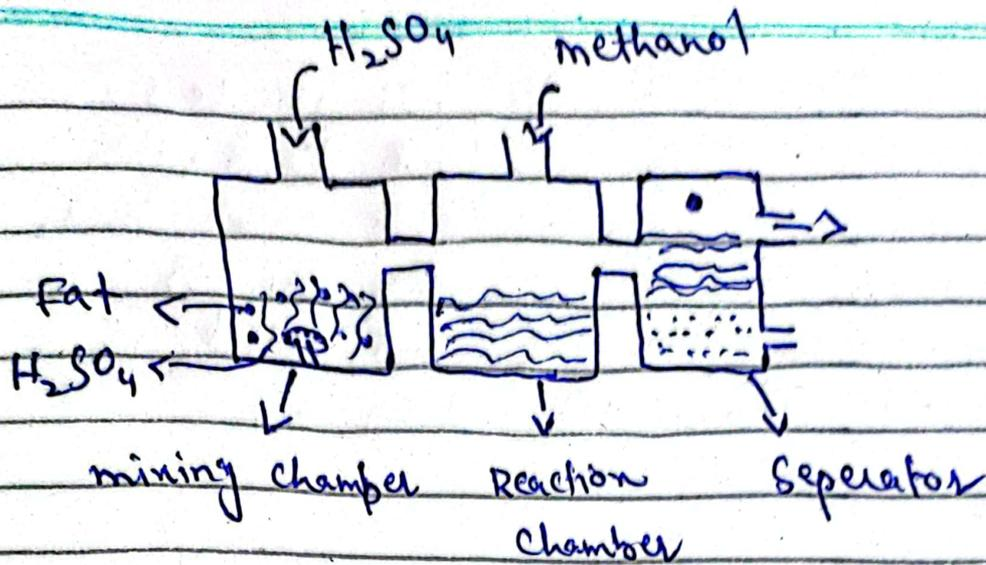
In mixing chamber we put ~~fat~~ fat and  $H_2SO_4$  and start the mixing chamber. The blade place in mixing chamber cut the fat into small peices and move it to reaction chamber. It is reaction chamber where maximum oil extraction take place. In separator all the other material stay at the bottom and oil stay at the top of the chamber. After the oil will be taken out and do further redefinement- we will add standard diesel in it.
