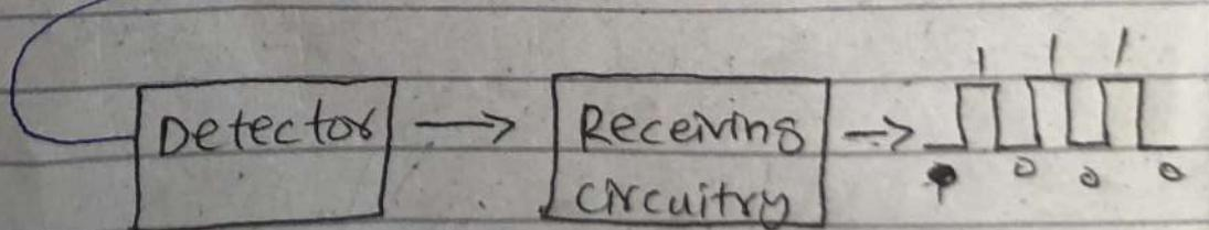
The receiving circuit consists of a photo detector, which is capable of measuring magnitude, frequency and phases of the optic field. Both LED and Laser can be used as a light sources based on the application.
